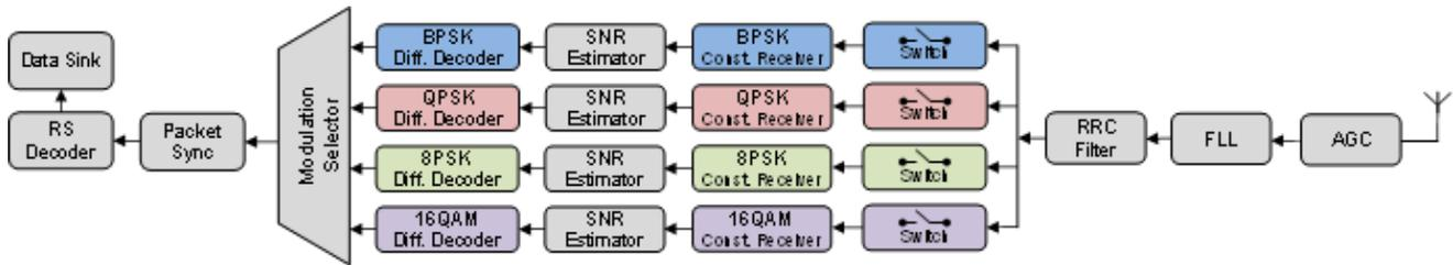
**Figure 5. Receiver of the WBR system**
