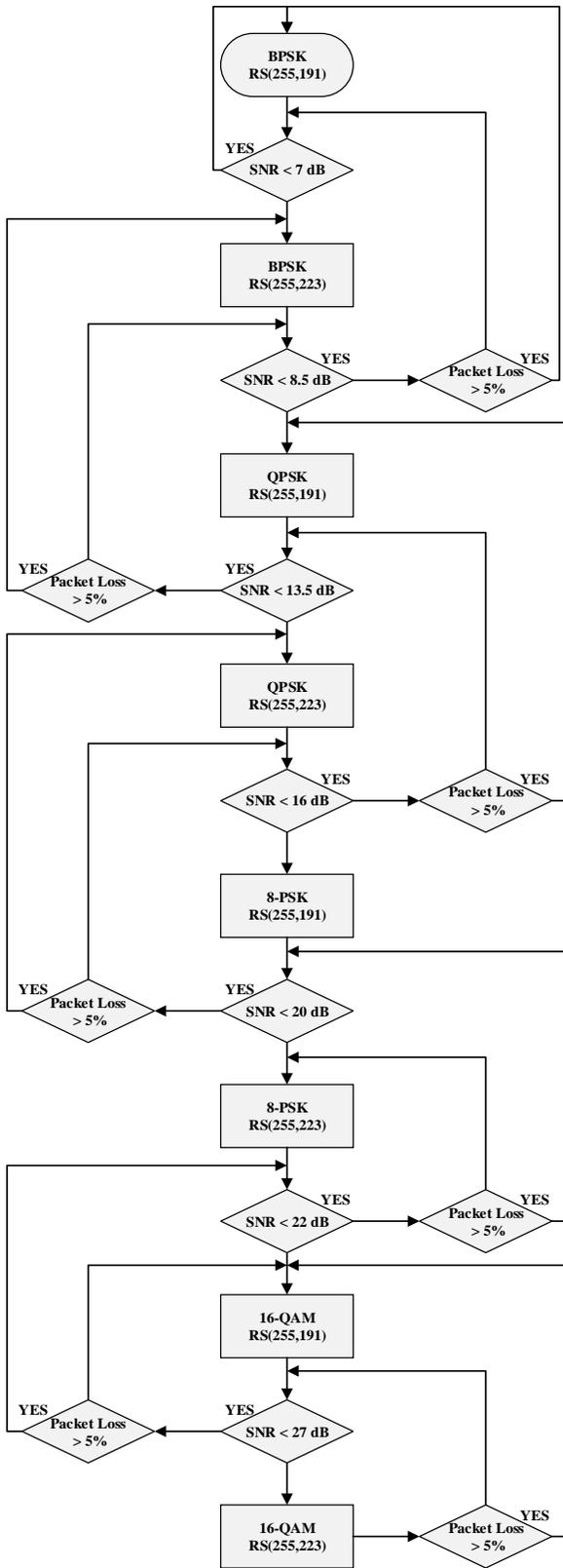
**Figure 3. ACM's switching scheme**
