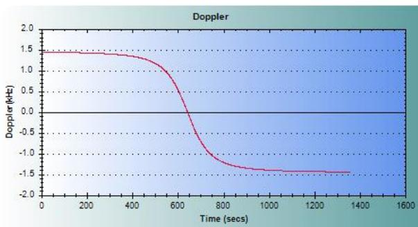
Figure 8. Doppler effect versus time of A/G link
