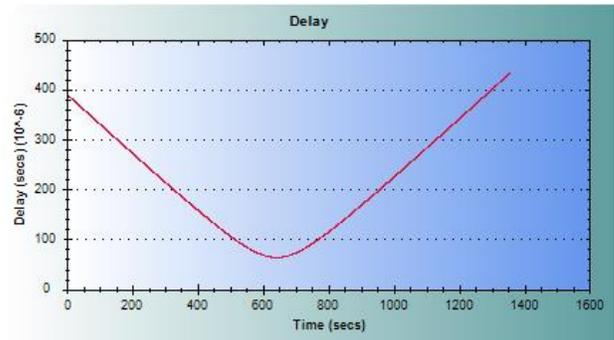
Figure 9. Delay versus time of A/G link
