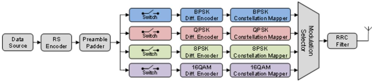
**Figure 4. Transmitter of the WBR system**
