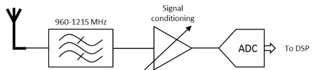
**Figure 1. Software Defined Radio Architecture**
