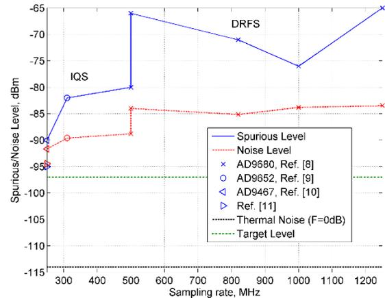
**Figure 2. State-of-the-Art ADC Performance**
