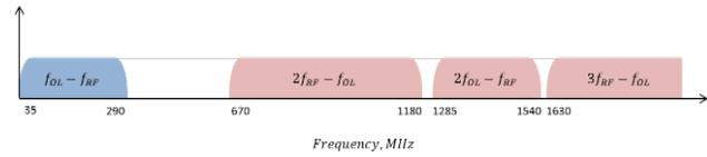
**Figure 4. Spectrum at the Output of the Mixer**
