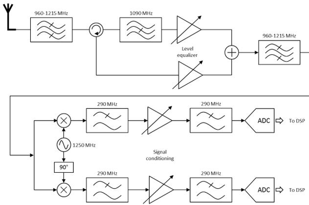
**Figure 3. Receiver Architecture**
