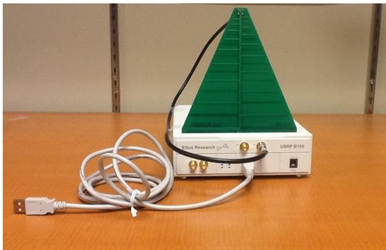
Figure 2: Photo of the SDR hardware (USRP B-100 equipment and antenna used for Mode S transponder prototype
