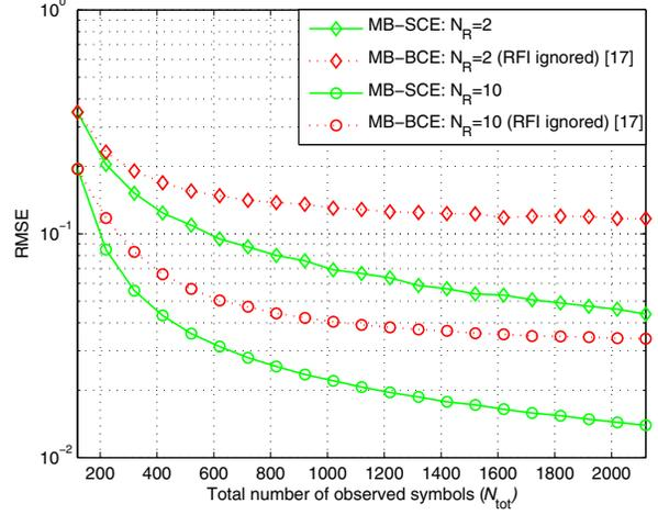
Fig. 2. RMSE performance of MB-SCE and MB-BCE for  $W = 10, L + 1 = L_f + 1 = 3, \text{SINR} = 10 \text{ dB}, \text{INR} = 10 \text{ dB}$  and  $N_{\text{tot}} = WN$ .
