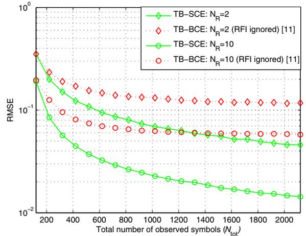
Fig. 3. RMSE performance of TB-SCE and TB-BCE for  $W = 10, L + 1 = L_f + 1 = 3, \text{SINR} = 10 \text{ dB}, \text{INR} = 10 \text{ dB}$  and  $N_{\text{tot}} = WN$ .
