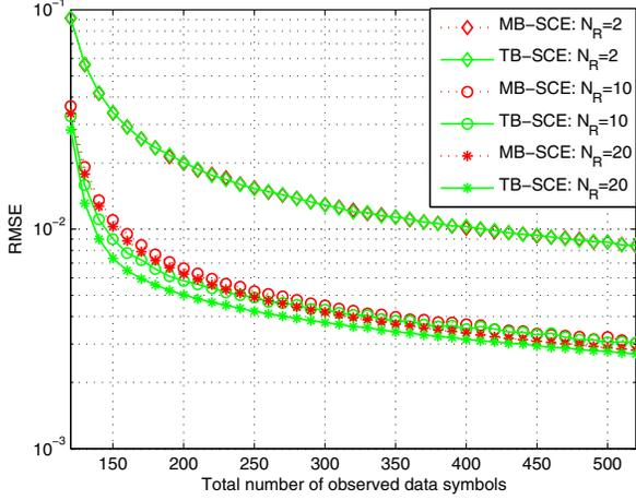
Fig. 4. RMSE performance of MB-SCE and TB-SCE for  $W = 10$ ,  $L + 1 = L_f + 1 = 3$ ,  $\text{SINR} = 30$  dB,  $\text{INR} = 5$  dB and  $N_{\text{tot}} = WN$ .
