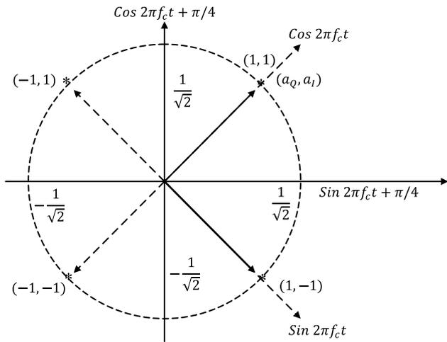
Fig. 3 Signal space diagram for QPSK and OQPSK.
