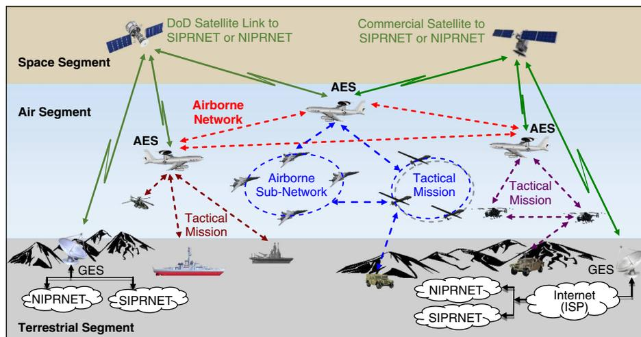
Fig. 2 Network architecture of global information grid (GIG).
