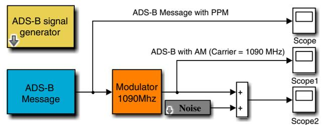
**Fig. 6 ADS-B generator and modulator.**
