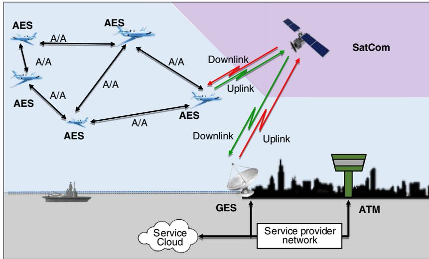
Fig. 1 Overall end-to-end system architecture for CAN satcom.
