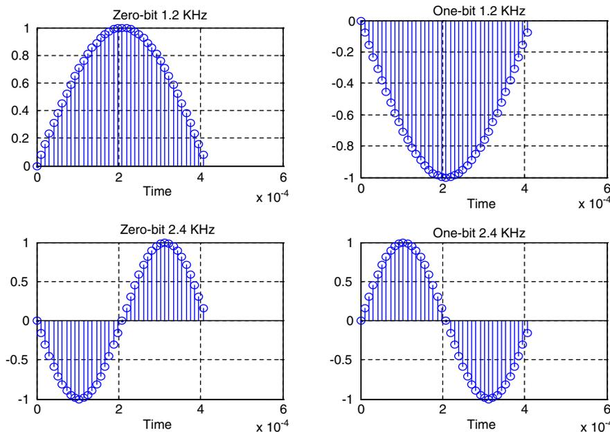
Fig. 4 Waveform from MSK modulator.
