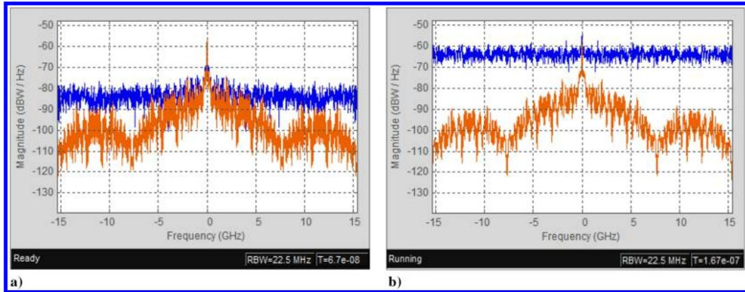
Fig. 11 Spectral density of A/A block for a) SNR = -20 dB; b) SNR = 20 dB.
