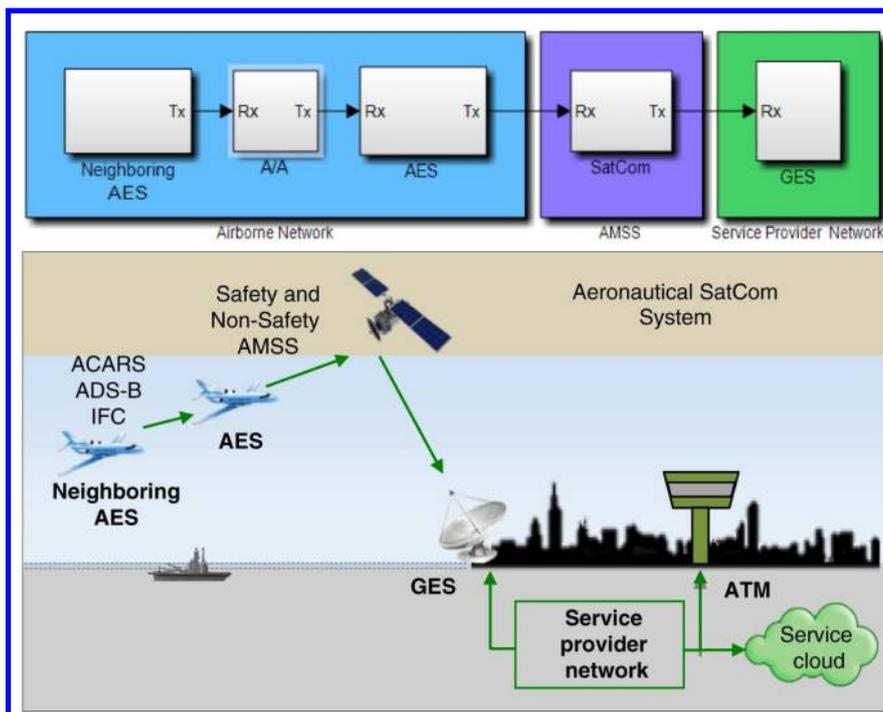
Fig. 8 Simulation architecture and scenario.
