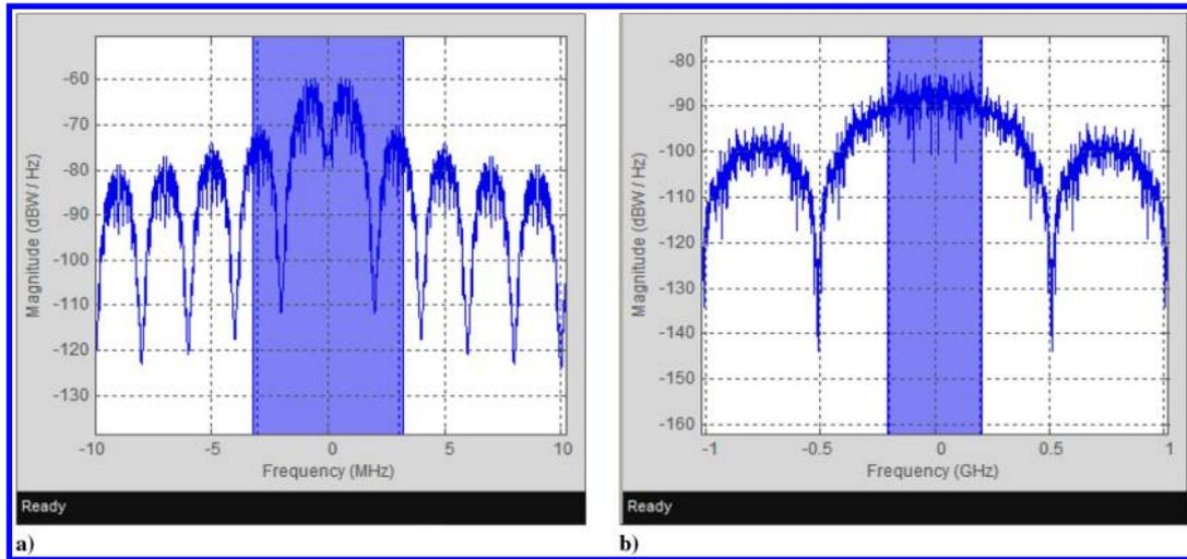
Fig. 12 Spectral density of a) NAES ADS-B generator; b) product of NAES ADS-B and Gold code 4.
