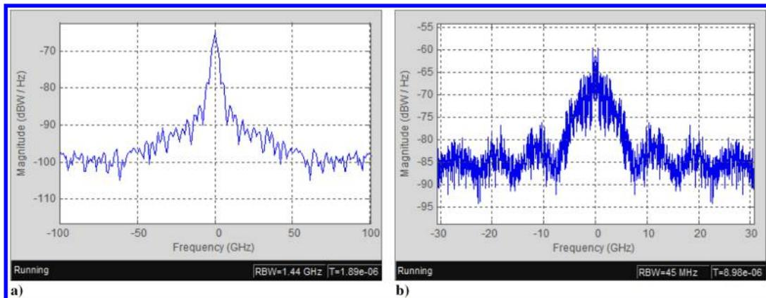
Fig. 13 a) Spectral densities in GES receptor for SNR = 10 with SF = 256. b) Spectral densities in GES receptor for SNR = 10 with SF = 8.
