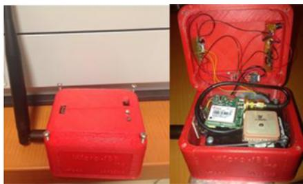
Figure 11. Data collector (Micro-iBB).
