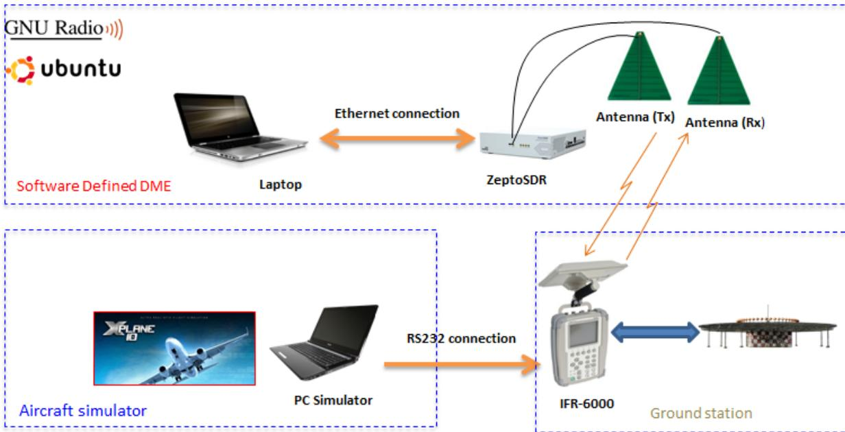
**Figure 2. Lab Test Bench Platform**
