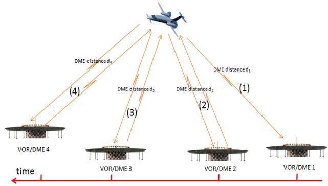
Figure 1. Sequential DME/DME Principle of Operation
