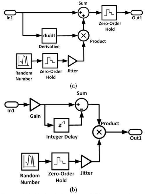
Fig. 5: Jitter model, (a) classical model, and (b) an appropriate model for NRZ feedback DAC.
