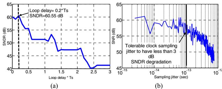
Fig. 7: SNDR versus (a) loop delay, and (b) clock sampling jitter.
