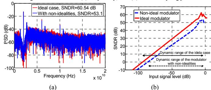
Fig. 8: (a) Output power spectral density, and (b) dynamic range of the BP CT-DSM.
