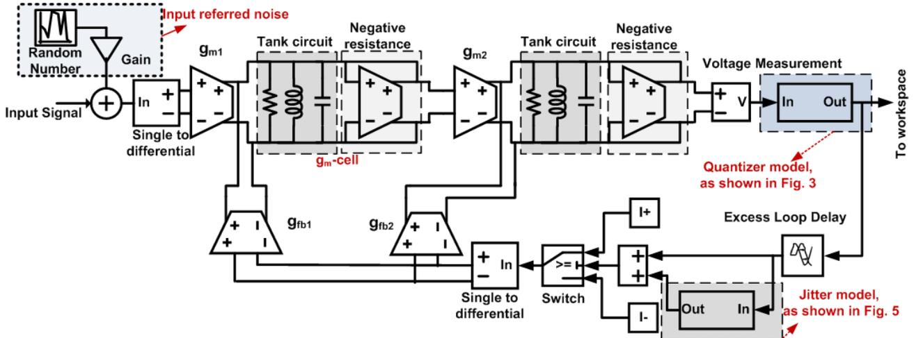
Fig. 6: Diagram of the BP CT-DSM with feedback structure.
