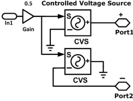
Fig. 1: Single-ended signal-domain to differential physical-domain interface diagram.
