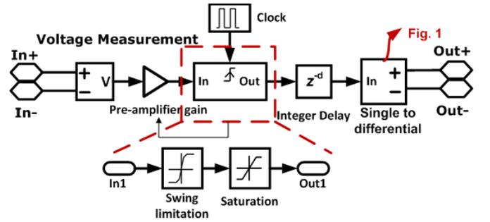
Fig. 3: Quantizer model.
