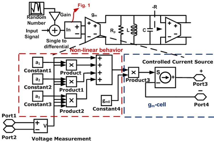
Fig. 2:  $g_m$ -LC resonator schematic.
