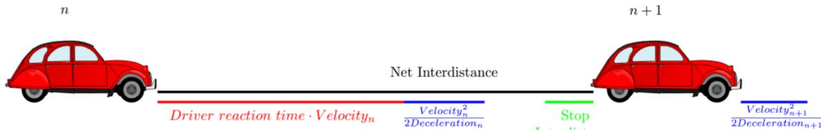
Figure 1. Important parameters related to driver safety evaluation in case of car following driving
