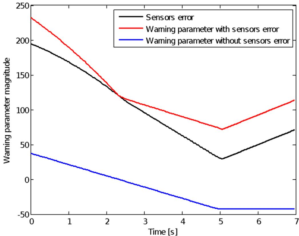
Figure 2. Impact of sensor errors on driver safety level using the PICUD indicator
