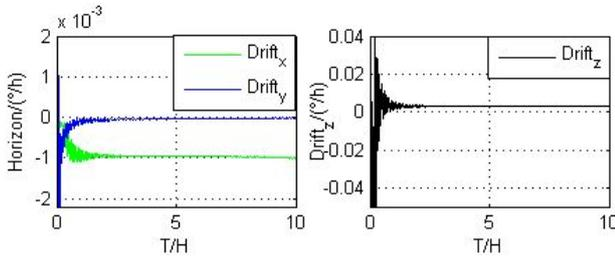
Fig.5: The estimate curves of gyroscope drifts
