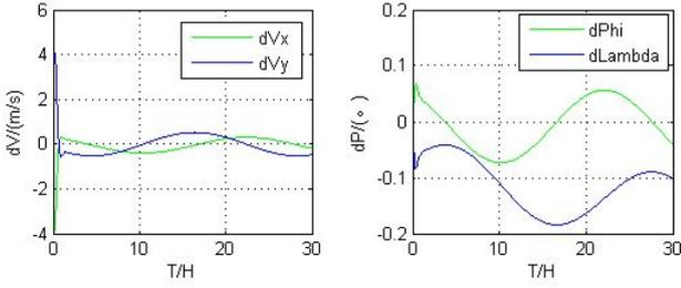
Fig.4: The error curves for SRINS working on the level damping mode
