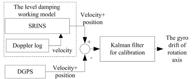
Fig. 2: The basic diagram of comprehensive calibration for SRINS
