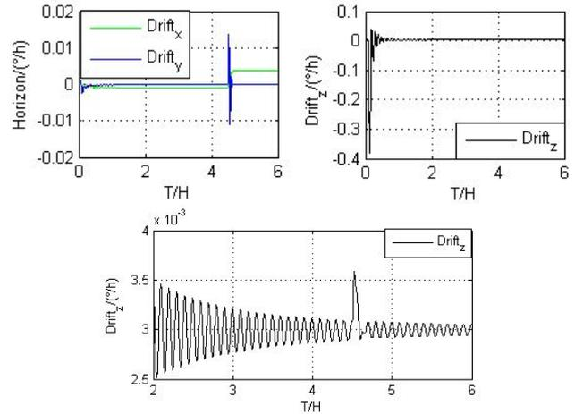
Fig.7: The estimated curves of gyroscope drifts with maneuvering in the steady state period
