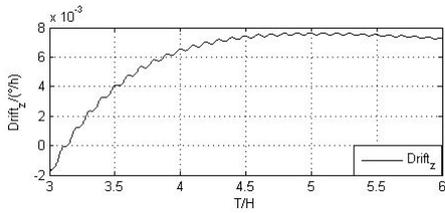
Fig.8: The estimate curves of gyroscope drifts with maneuvering in the initial period
