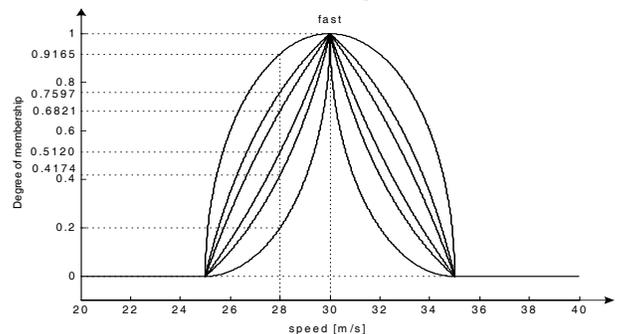
Fig. 5. The elliptical membership function.
