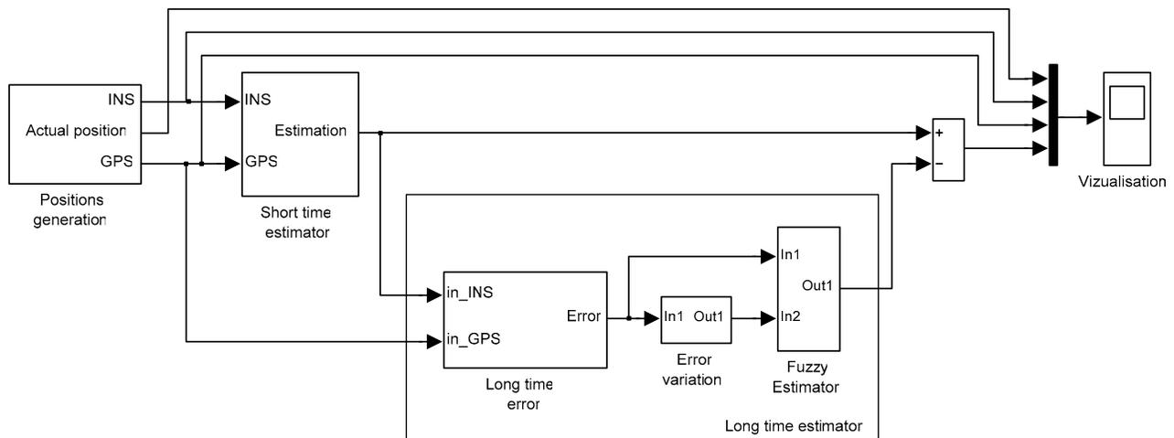
Fig. 6. The system used to enhance GPS/INS synergy.
