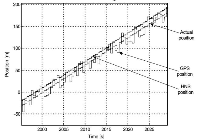
Fig. 12. Zoom into the positions reported by GPS and HNS, as well as the actual position.
