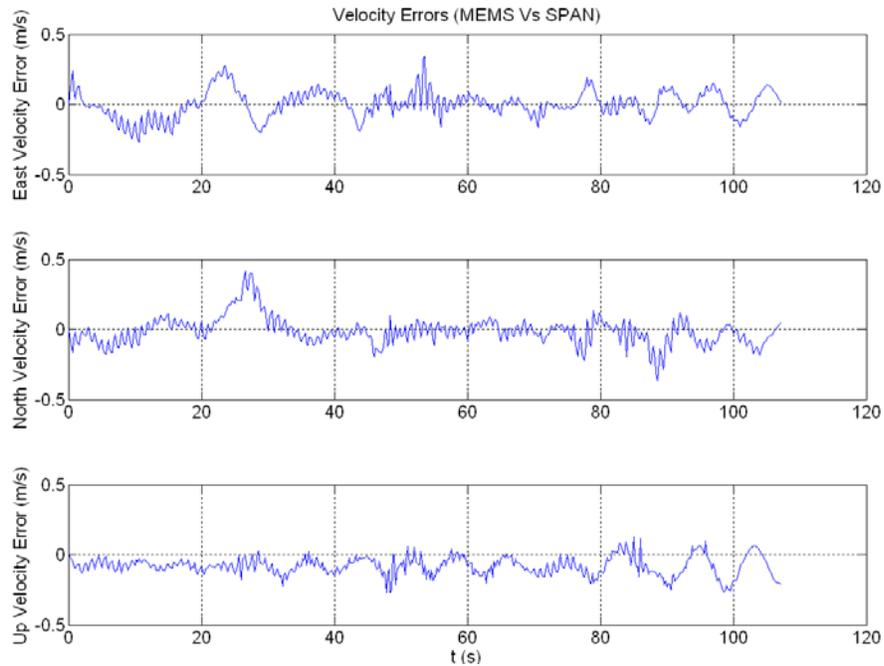
**Figure 7: Velocity Errors (East, North and Up) (MEMS vs SPAN)**
