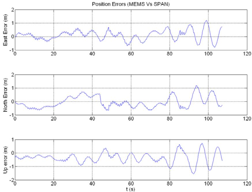
**Figure 6: Cartesian Position Errors (latitude, longitude and altitude) (MEMS vs SPAN)**
