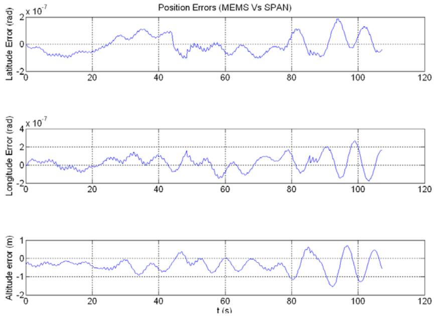
**Figure 5: Geographic Position Errors (latitude, longitude and altitude) (MEMS vs SPAN)**
