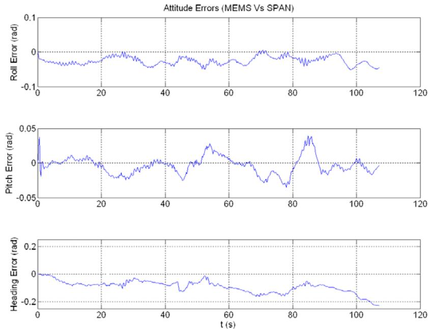
**Figure 8: Attitude Errors (Roll, Pitch and Heading) (MEMS vs SPAN)**
