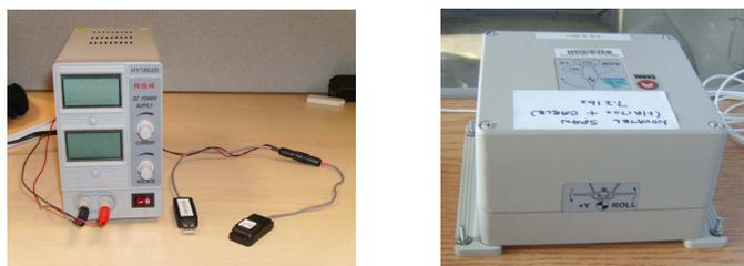
Fig. 4 nIMU MEMS sensor and SPAN IMU
